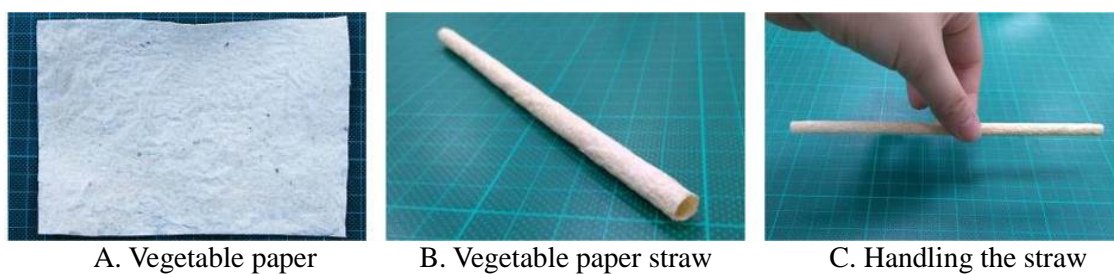
Figure 2. Finished product of the vegetable paper and vegetable paper straw.
