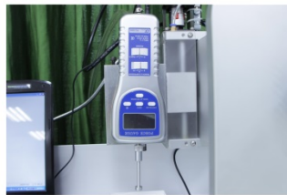
Force Gauge Lutron FG-5005 (Taiwan)
