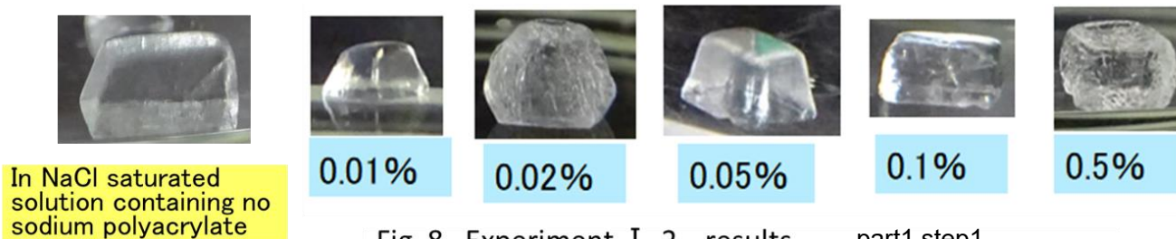
Fig. 8 Experiment I -2 results part1 step1 value: mass percentage concentration of sodium polyacrylate
