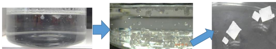
Fig.4 generated crystals in the supersaturated NaCl aqueous solution with 4% sodium polyacrylate
