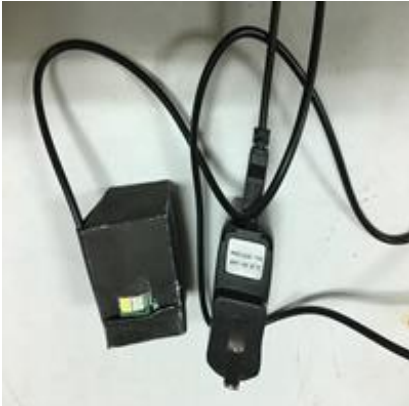
組裝好 5V LED 電源光源盒後備用
